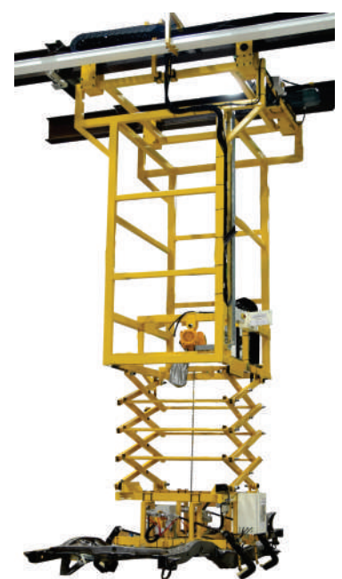
Transfer of frames from one fixtures to another in a automotive welding line
